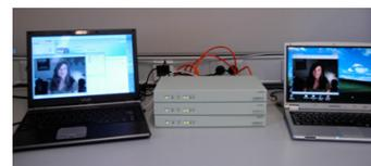
Figure 4. ARP-Path Switches network with Soekris (Linux) boards
